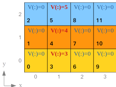
Figure 42 – Broadcast of a V array in the degenerated 2D grid.
