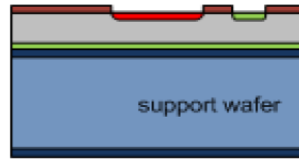
d) Oxide growth, lithography, etching and ion implantation to form doped regions
