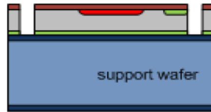
e) ICP etching to reveal the edge
