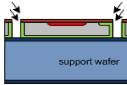
f) Four-quadrant ion implantation to activate edges
