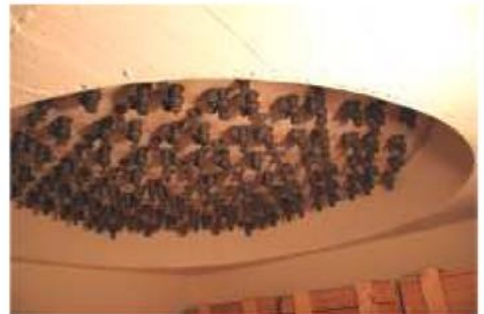
Fig. 12. The complex mechanism of 183 screws to regulate the 61 tiles can be seen on the ceiling of the small room placed under the 1.80 m mirror. (photo: F. Bonoli)
